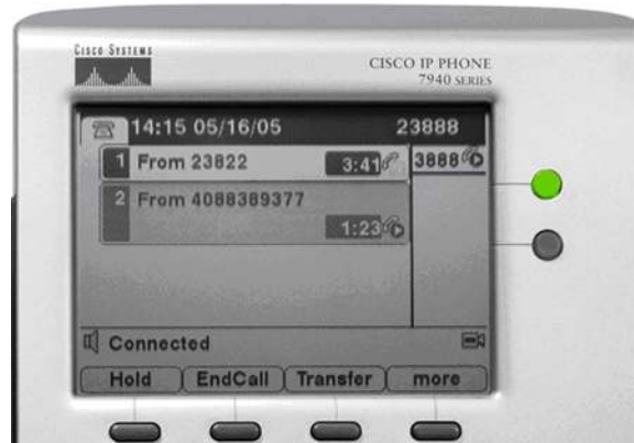
Figure 2. Close-Up of High-Resolution Display and Lighted Line Keys
